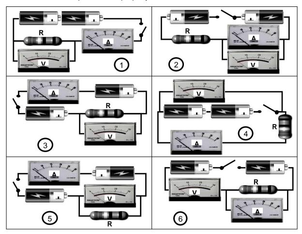
1.1 Identify TWO circuits in which the components are CORRECTLY CONNECTED to carry out the investigation. Write down ONLY the numbers of these circuits.
